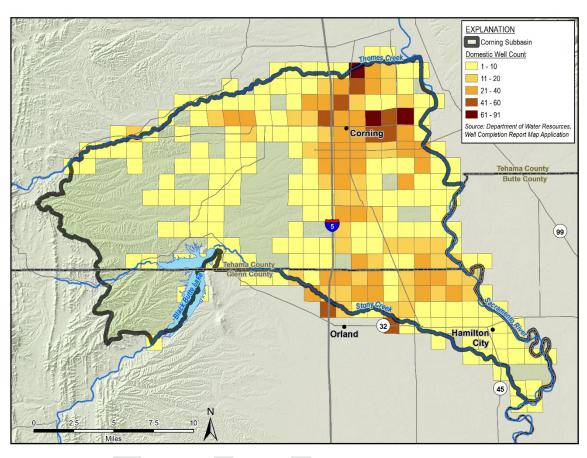
Figure 2-12. Density of Domestic Wells (Number of Wells per Square Mile)<sup>14</sup>
